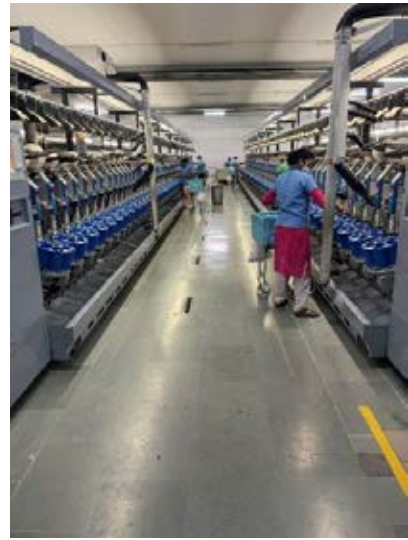
Production Process - winding.JPG
